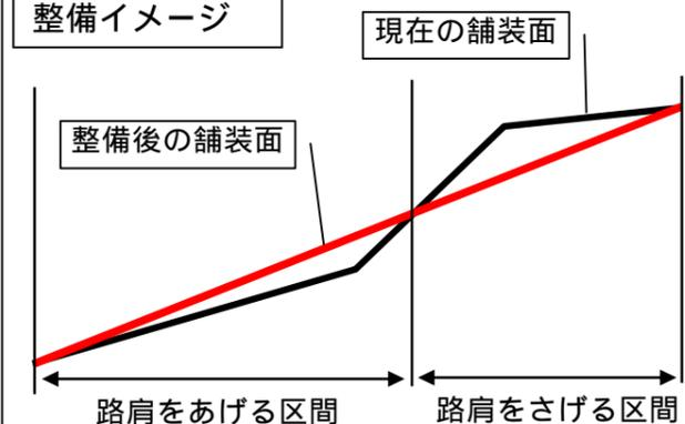
沿道の方と調整し、可能な限りうねりを解消 (Adjust with the road side and eliminate ripples as much as possible)
